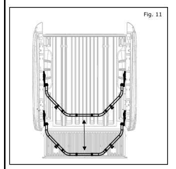
12) When the Bed Extender is at the further rear position, push down on the buckle to insert into tailgate latch. Tighten straps. To release, pull tailgate handle.
