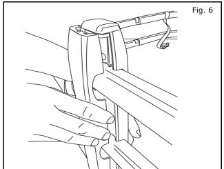
6) Attach plastic upright around the tube juncture (like a sandwich), placing a rubber bumper into the two ends of the upright. (figure 6)
