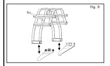
**NOTE:** Sliding Bed Extender comes pre assembled and ready to drop into vehicle
