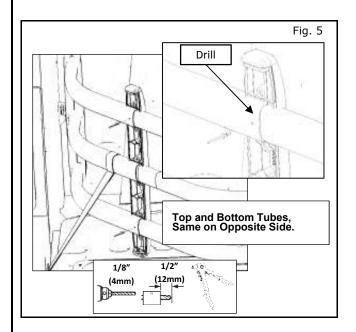
5) Use a 1/8" drill bit to drill a Hole into top and bottom center tubes to allow for pivot tube and center tube to be riveted together. (This is shown in figure 5)
