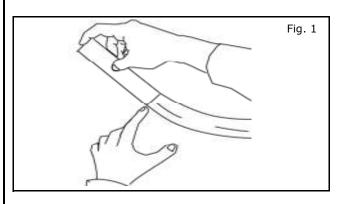
1) Note the unpainted section of the tubes. This will be used as a guide to assemble the tubes together. Figure 1 shows the intersection point of the center tube.
