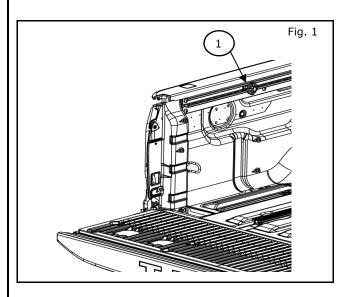
1) Wipe away any dirt or debris from inside surfaces of Utility-Track C-Channels
