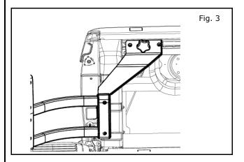
4) To secure the Sliding Bracket Assemblies position on the C-channels, turn the knob clock-wise until it bottoms against the C-channel, Tightining knobs should be torqued to a range of 3.4 N-m to 5.6 N-m or 30 in-lbs. to 50 in-lbs.
