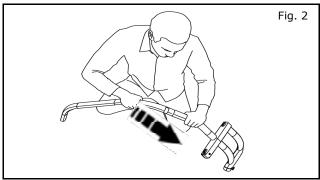
2) Slide the center tube into the center tube of 3-tube assembly (figure 2). Do this for the following tubes shown in figure 3.
