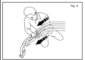
4) To keep tube overlap constant, adjust each tube equal on all sides. (figure 4)
