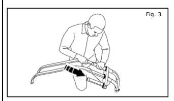
3) Insert the bottom long tube into the bottom tube of the 3-tube assembly as shown in figure 3 and 4. Repeat for the other side.
